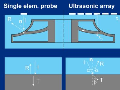
Normal incidence transmitted and reflected wave intensities
