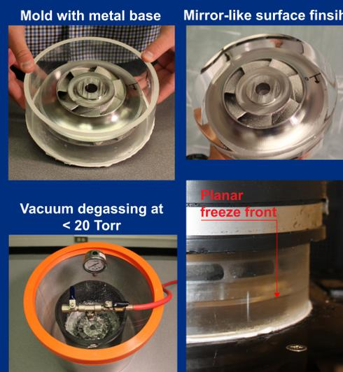
Freeze front propagation model at constant cold plate temperature
